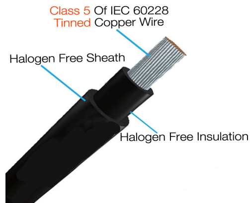
Fig 5.1 DC Cable cross section | Clare solar
