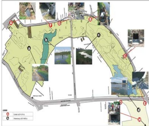
It was found that most of the sewers were transporting high loads of wastewater, with pollution levels much higher than CPCB permissible limits. Based on our recommendation. The entry of wastewater into the poonga was arrested in collaboration with CMWSSB. A 'POLLUTION WATCH' was initiated to continuously monitor the flow in outfall.
