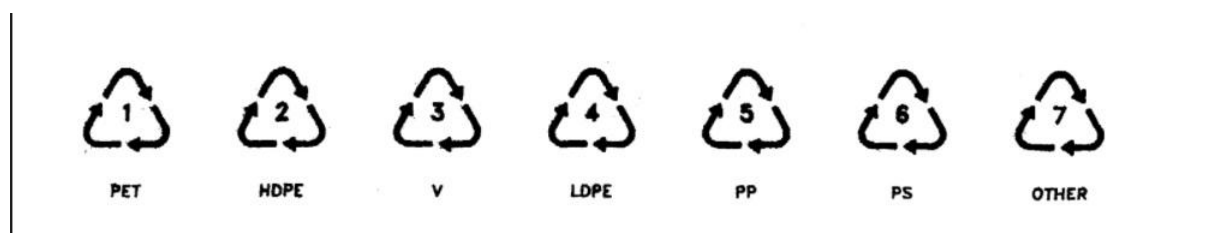
Figure 1: The symbols that should be used by the manufacturers to print on the plastics they use (Source: Guidelines for Recycling of Plastics, IS 14534 (1998))
