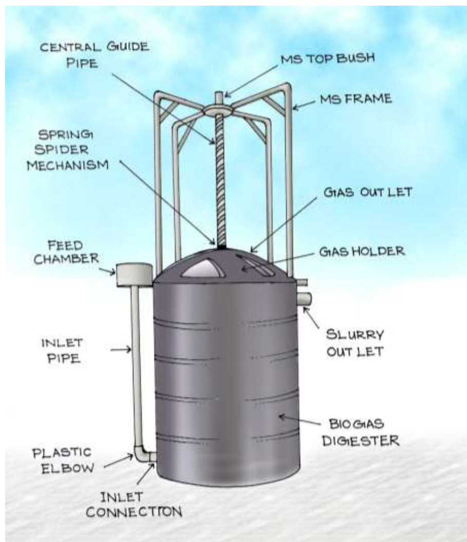
Figure 28: A typical household biogas plant
