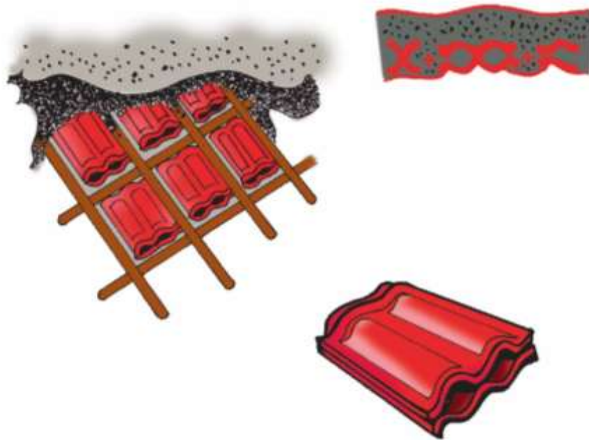
Figure 14: Filler slab with hollow blocks or double layered Mangalore tiles
