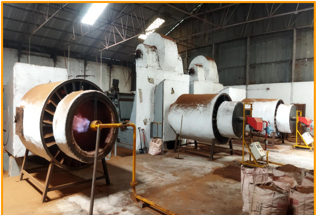
Fig 2.13 : Tea Dryer : E C P Type : Front View and Back View | CAG
