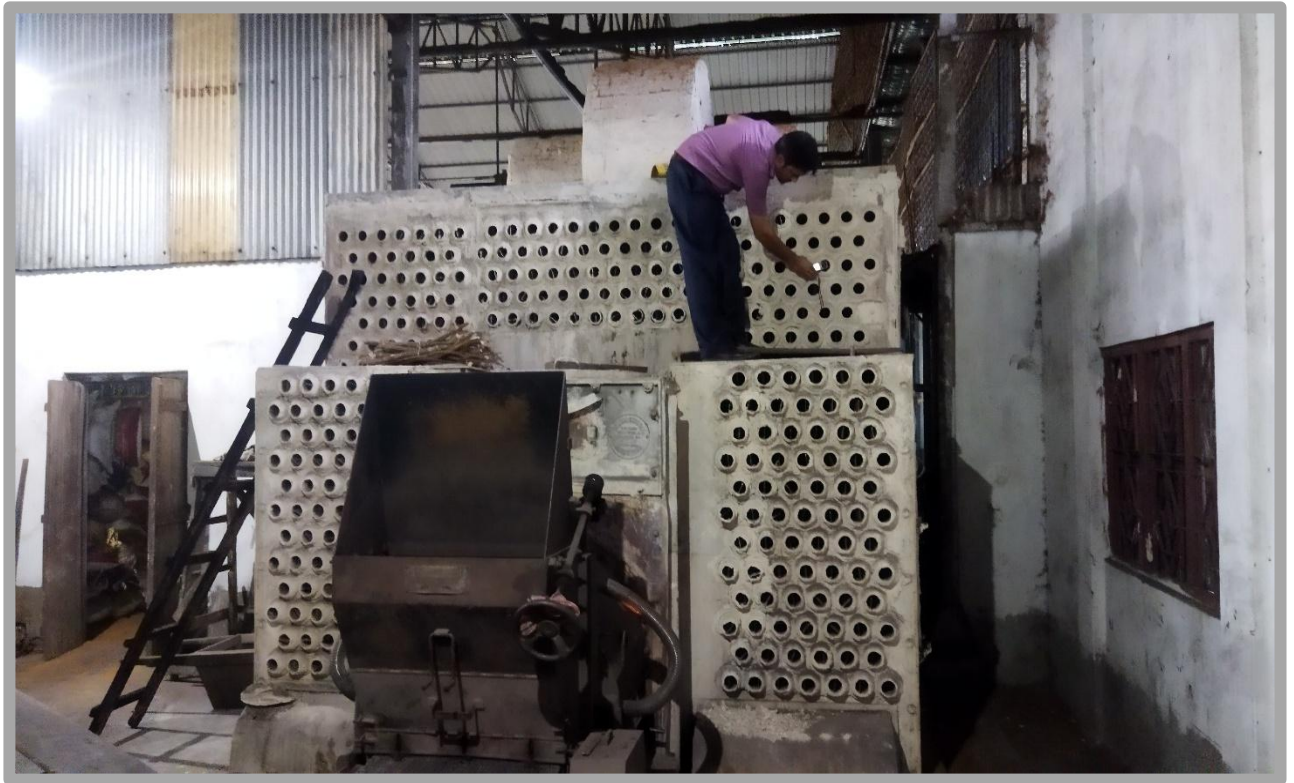
Fig 2.11 : Tea Dryer : Furnace : Frontal View | CAG
