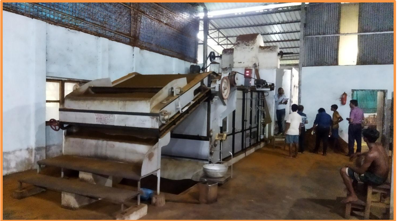
Fig 10.5 : Tea Dryer : E C P Type: Frontal View | CAG
