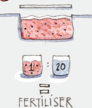
When leachate collection tank is full, remove the leachate. Dilute with water in 1:20 ratio and use as a fertilizer.
